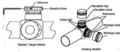
Your Osprey scope has precise windage (left and right), elevation (up and down), and adjustments, with audible and tactical clicks. The click value is 1/4 MOA for hunting models and 1/8 MOA for tactical/varmint models. You can find click value for your scope marked on the windage/elevation knob. The following table will be useful when zeroing (described later in the manual) or making adjustments in the field.
