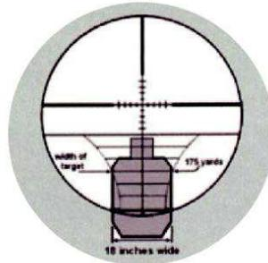
After bracketing the target in the choke, count the number of lines down the choke to determine the target distance. The top line is equal to 100 yards with each line below being further in 25 yard increments. (ILL. 2)
