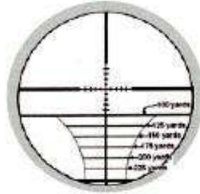
The “choke” lines are not intended to be used as a ballistic reticle. This portion of the reticle is only intended for the range estimation of an 18 inch target. After “ranging” you target, make the appropriate adjustments to the Bullet Drop Compensator (BDC) if equipped on your scope, or adjust your scope’s elevation to compensate for the bullet drop at the determined range.
