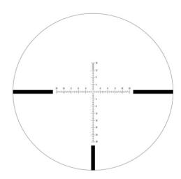
A ES MOA reticle is named for the linellae and spaces it is composed of . The space between the linellae is one moa, and the middle of "+"will be red/green/blue illumination. This arrangement is very useful for determining the distance of objects of a known size, the below chart will be huge help.
