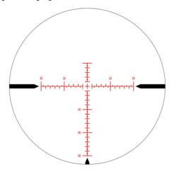
The L-MOA reticle is a simplistic reticle that allows to do holdovers with ease. Each hash is equal to 1 MOA. A hash with the number 5 is equal to 5 MOA's. A MOA is a unit of angular measurement, like degrees or minutes of angle. A MOA is equal to 1 inch at 100 yards (at any zoom). On the next page you will find a more detailed overview of the reticle
